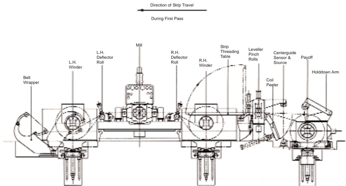
Due to the demands set forth by the stainless steel industry for better quality strip, Waterbury Farrel® made another revolutionary change in the traditional monoblock Z-Mill® Rolling Mill by including bottom power crown control and by substantially increasing the mass of the housing to achieve higher mill rigidity. The mill (colored graphic) can roll stainless strip of 0.1mm thick and 1300mm wide at very high speeds while maintaining close tolerances. Advantages of this design include:
